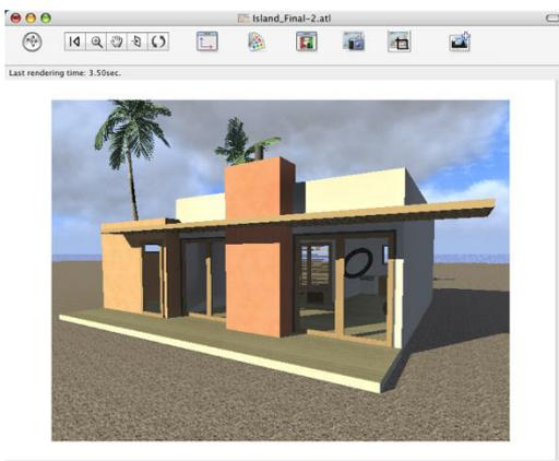
Both the toolbar commands (Navigation, Zoom, Pan, Front View) and the Keyboard and Mouse Shortcuts specific to the Preview window are used to navigate within a scene.
